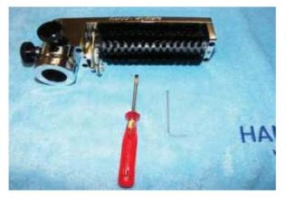
The package contains an Allen key to set up the rotary brush and a screwdriver to reposition or replace the rotary brush.
