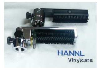
Locate the rotary brush over the brush socket and push the brush down until the brush sits between one and two millimetres above the disc.. Fix in place with the rear thumb screw. Optional mounting socket (rotary brush extension set) Already assembled with the ELB and B devices.
