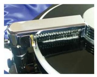
To achieve optimal cleaning results change the direction in which the disc is rotated from time to time.
