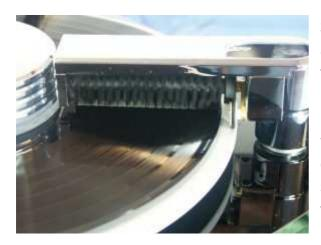
Select the lowest speed to start the Mera, Micro and Aragon EL models. With the ELB models use the "Brush" button. Loosen the thumbscrew and push the brush down only so far that is makes light contact with the disc surface. Relock the arm with the thumb screw. The arm is now in the correct position. If the brush bristles bend and spray cleaning fluid then you have set the brush too close to the disc..
