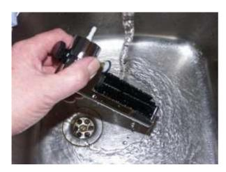
After using the rotary brush we recommend a thorough rinsing with warm running water, after which the brush should be wiped dry with the supplied microfibre cloth These simple steps will ensure trouble free usage of the rotary brush.
